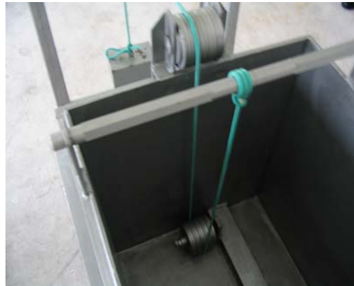
Photo 1a. Trough for a preliminary testing of high explosives (inside view)
