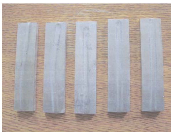
Photo 4 Witness plates with the indentations produced by the detonating cord RIOCORD 6g/m ANTIGRISU after immersion in water for 24 hours under a traction force of 402N.
