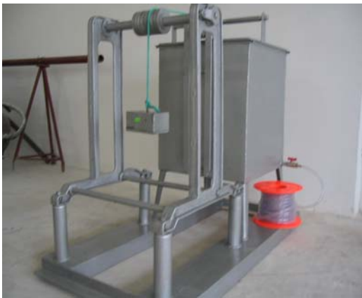
Photo 2. Stand for testing waterproofness detonating cords
