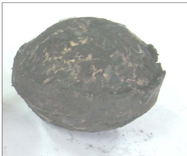
Figure 3. Bricks with coal sludge, oil coke, sawdust, Ca (OH) 2 and molasses
