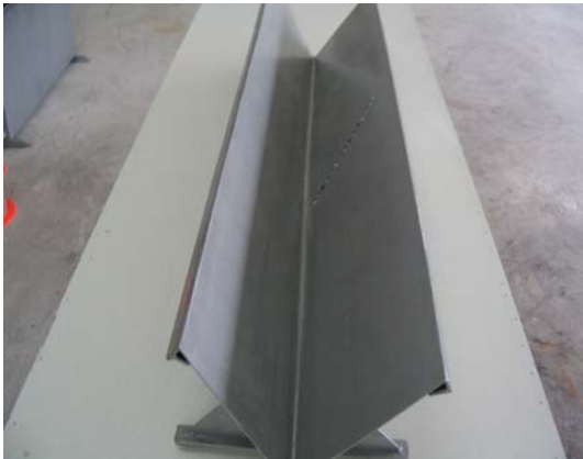
Photo 1a. Trough for a preliminary testing of high explosives (inside view)
