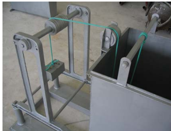
Photo 2. Stand for testing waterproofness detonating cords
